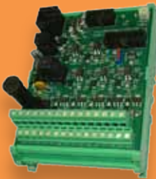
NMEA expansion module for VDR link incl. selector for back-up OOW cabins alarm transfer & emergency call NMEA 210.24.0.0
